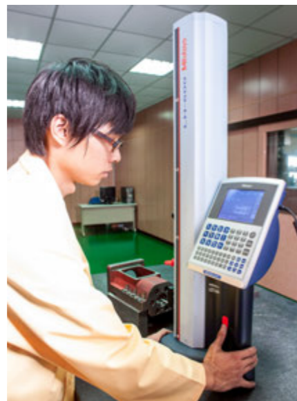
Measurement of inspection by 2D coordinate 2D
